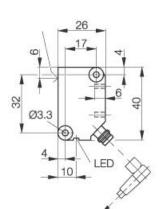
Inductive Sensors BES R05KB-POC40B-S49A 12 x 40 x 26 normally-closed Sn=4mm shielded
